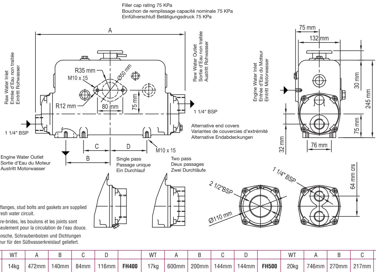
Engine inlet and outlet flanges have identical dimensions.
