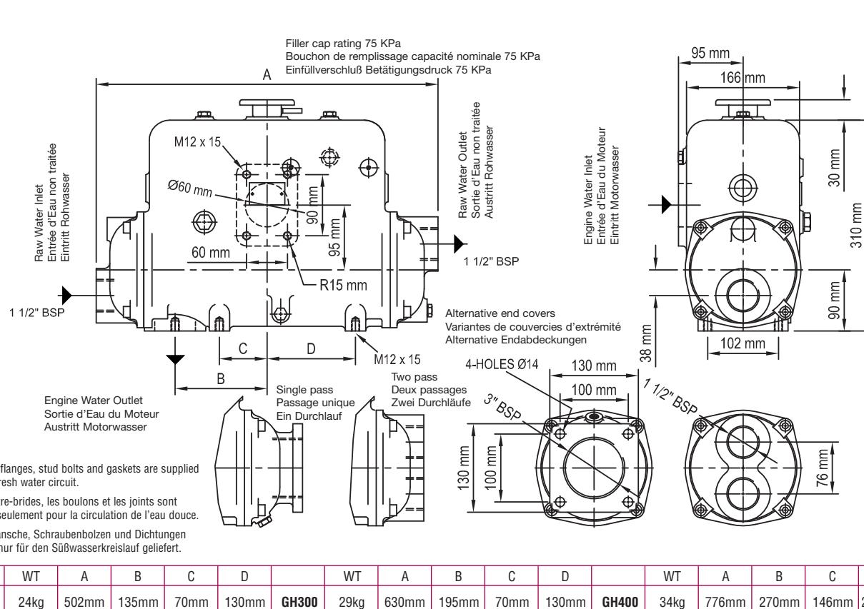
Engine inlet and outlet flanges have identical dimensions.
